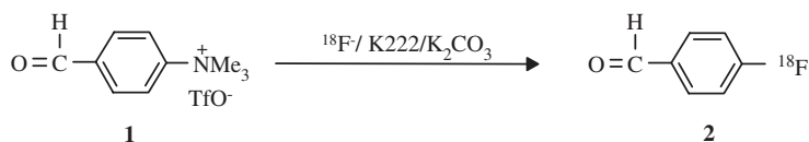
Scheme 2. Synthesis of 4-[ ^{18}\text{F} ]fluorobenzaldehyde (2)
